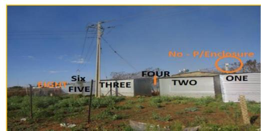
An average, 8 shacks per formal RDP house can be observed in Pimville Zone 9. Instead of supplying the original 2,000 RDP dwellings, the network now supplies 16,000 dwellings. The network originally designed for 4MVA is made to supply 32MVA load. This situation gives rise to the following consequences;
