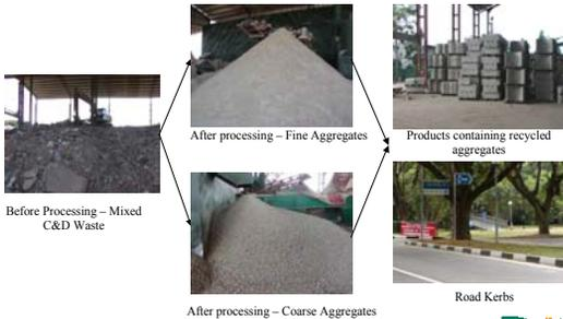
...Construction & Demolition Waste Recycling
